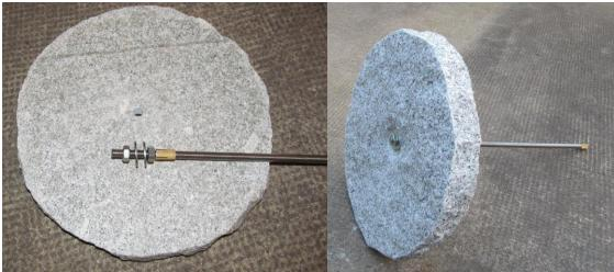
Fix the second brass expansion anchor at the top of the threaded rod, allowing it a little bit expansion (just so much that it fits into the tube tightly)
